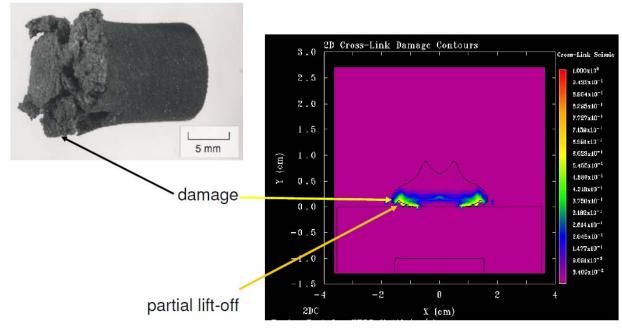
Taylor test coupled damage and reactivity model experiment and numerical prediction
